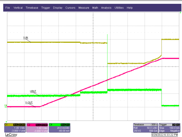
Figure 8-9. ISET Short-Circuit Response
