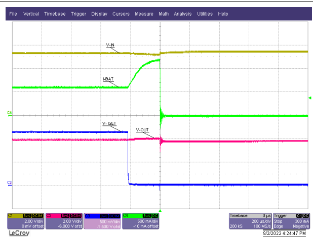
Figure 8-7. OUT Transient Response
