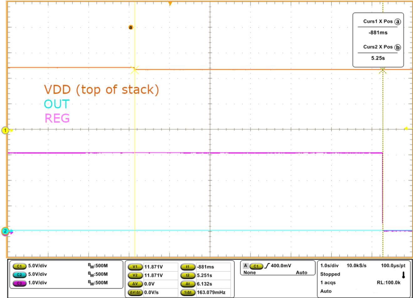
Figure 8-6. Undervoltage Detection to Disable the Regulator
