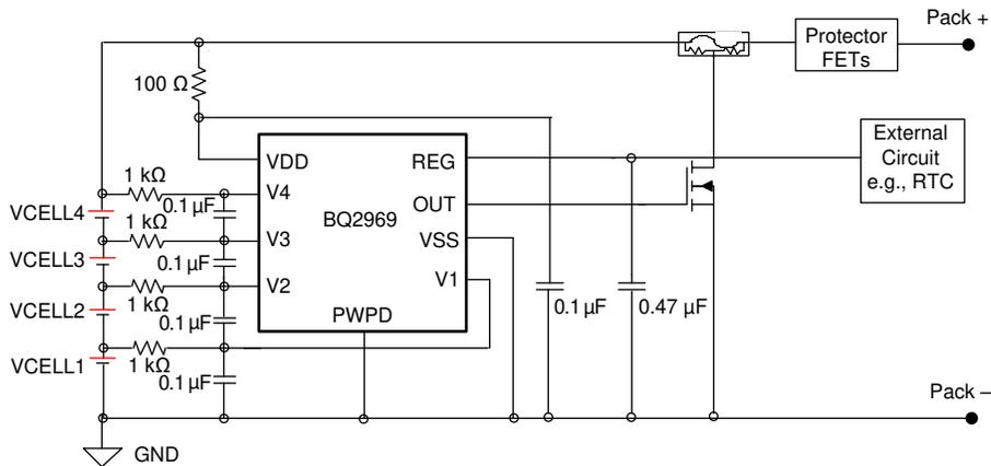
**Figure 8-1. BQ2969 4-Series Cell Typical Implementation (Simplified Schematic)**
