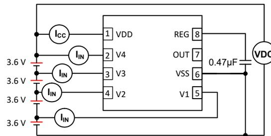
**Figure 7-5. Configuration for Integrated Circuit Current Consumption Test**
