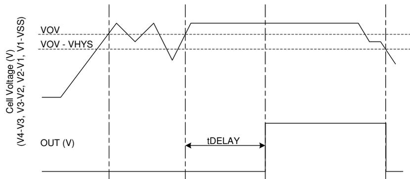
**Figure 7-2. Timing for Overvoltage Sensing for OUT**
