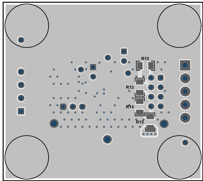
Figure 10-2. BQ2969 Two-Layer Board Layout - Bottom Layer
