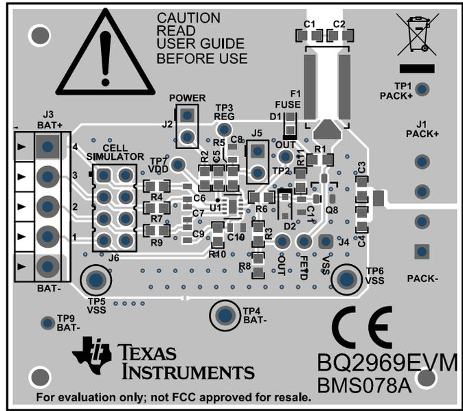
Figure 10-1. BQ2969 Two-Layer Board Layout - Top Layer
