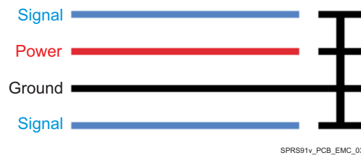
Figure 7-13. Guard Ring Routing
