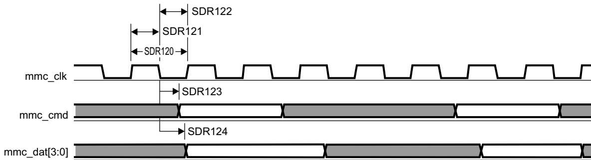
Figure 5-59. MMC/SD/SDIOj in - SDR12 - Transmitter Mode
