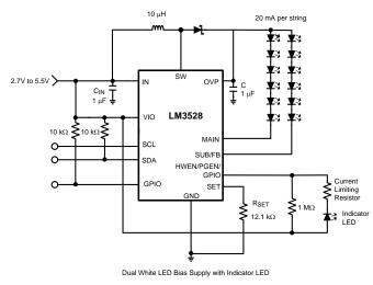
Figure 1. Typical Application Circuit
