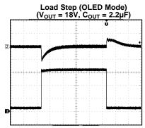
Channel 2: V<sub>OUT</sub> (AC Coupled, 500mV/div)
