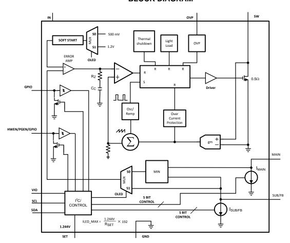
Figure 37. LM3528 Block Diagram
