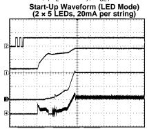
Channel 2: SDA (5V/div) Channel 1:  $V_{OUT}$  (10V/div) Channel 3:  $I_{LED}$  (20mA/div) Channel 4:  $I_{IN}$  (200mA/div) Time Base: 400 $\mu$ s/div
