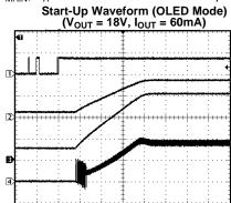
Channel 1: SDA (5V/div) Channel 2: V<sub>OUT</sub> (10V/div) Channel 3: I<sub>OUT</sub> (20mA/div) Channel 4: I<sub>IN</sub> (200mA/div) Time Base: 400µs/div
