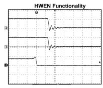
Channel 4: I<sub>SUB</sub> (20mA/div) Channel 3: I<sub>MAIN</sub> (20mA/div) Channel 2: HWEN (5V/div) Time Base: 200ns/div
