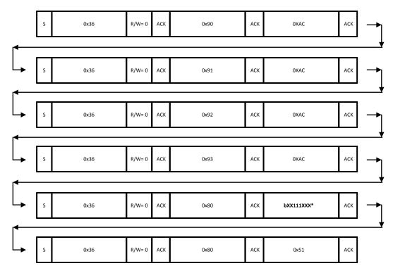
\*Only bits <5:3> are necessary in this byte the rest are don't cares. Bits <5:3> = '111' are necessary to latch the pattern generator data bits into the internal shift register.
