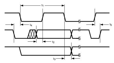
Figure 4. I<sup>2</sup>C Timing
