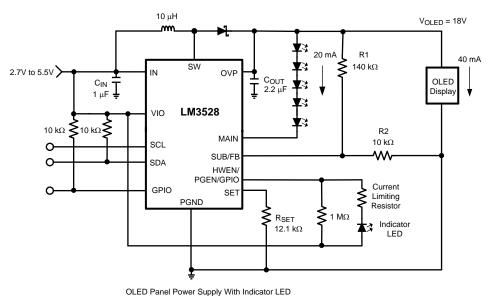
Figure 54. LED Backlight + OLED Power Supply
