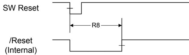
**Figure 18-9. Watchdog Reset Timing**
