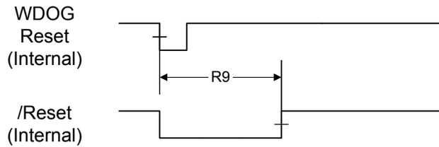
**Figure 18-10. LDO Reset Timing**
