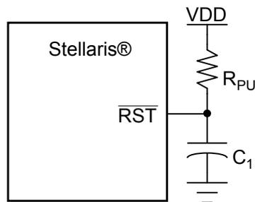
$R_{\text{PU}} = 1$  k $\Omega$  to 100 k $\Omega$
