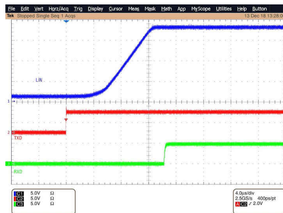
Figure 10-12. Dominant to Recessive Propagation Delay
