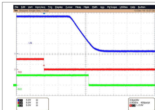
Figure 10-11. Recessive to Dominant Propagation Delay
