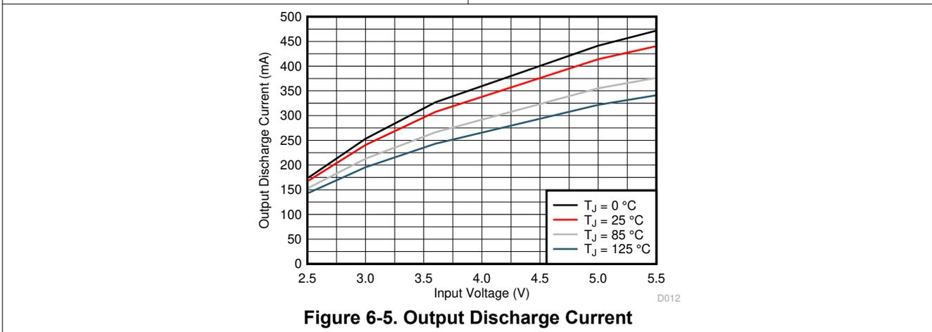
Figure 6-5. Output Discharge Current
