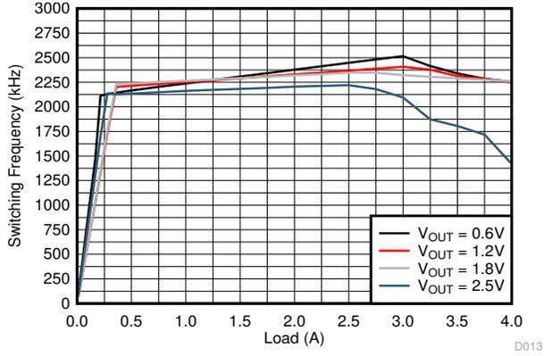
Figure 8-27. Switching Frequency
