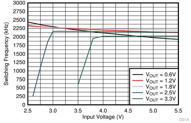
Figure 8-28. Switching Frequency
