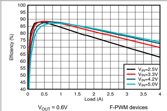
Figure 8-5. PWM Efficiency
