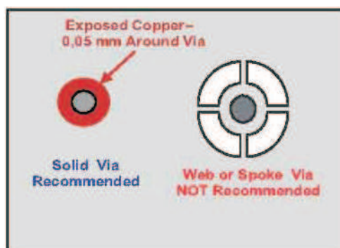
Figure 27. Thermal Via Connection at the Bottom Layer
