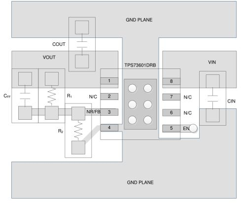
Figure 7-9. Adjustable Output Voltage Option Layout (DRB Package)
