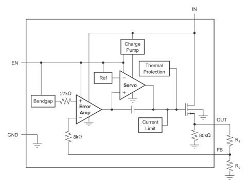
$$\begin{split} V_{OUT} &= (\ R_1 + R_2 \ ) \ / \ R_2 \times 1.204 \\ R_1 \ || \ R_2 &\cong 19 \ k\Omega \ \text{for best accuracy.} \end{split}$$
