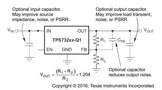
Figure 7-2. Typical Application Circuit for Adjustable-Voltage Versions
