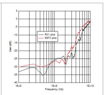
Figure 5-10. Input Return Loss Performance
