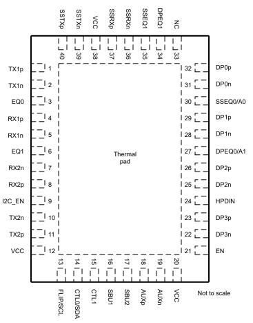
Figure 4-1. RGF Package, 40-Pin (VQFN) (Top View)
