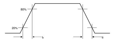
Figure 6-5. Output Rise and Fall Times
