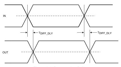
Figure 6-3. Propagation Delay
