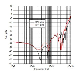
Figure 5-12. DisplayPort Output Return Loss Performance
