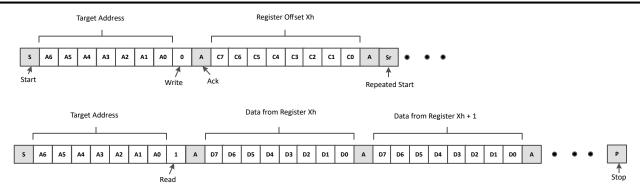
Figure 7-4. I<sup>2</sup>C Read with Repeated Start
