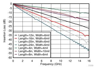
Figure 8-5. Insertion Loss of FR4 PCB Traces
