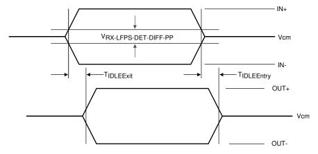
Figure 6-4. Electrical Idle Mode Exit and Entry Delay
