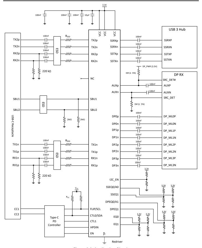
Figure 8-2. Application Circuit
