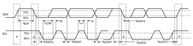
Figure 6-1. I<sup>2</sup>C Timing Diagram Definitions
