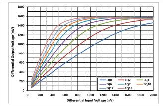
Figure 5-9. USB RX (UFP) Linearity Curves at 2.5GHz
