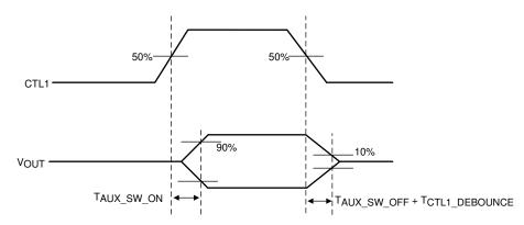
Figure 6-6. AUX and SBU Switch ON and OFF Timing Diagram
