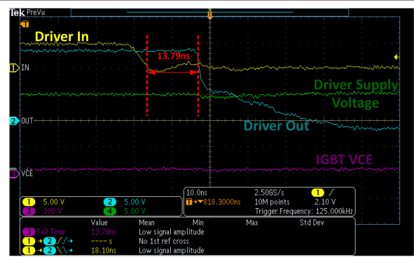
Figure 7-3. UCC27624-Q1 Used to Drive IGBT in the Boost Converter
