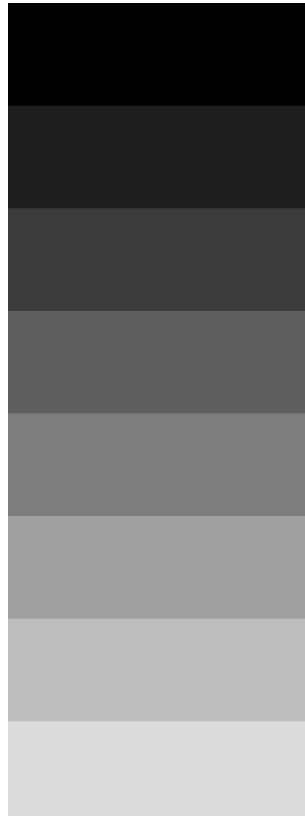
Figure 3-3. Example of Fixed Step Vertical Ramp Test Pattern
