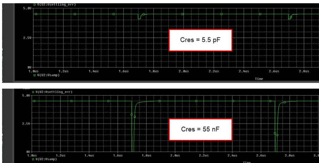
Figure 3-9. Output Settling With C_{res} = 5.5 \text{ pF} and 55 nF
