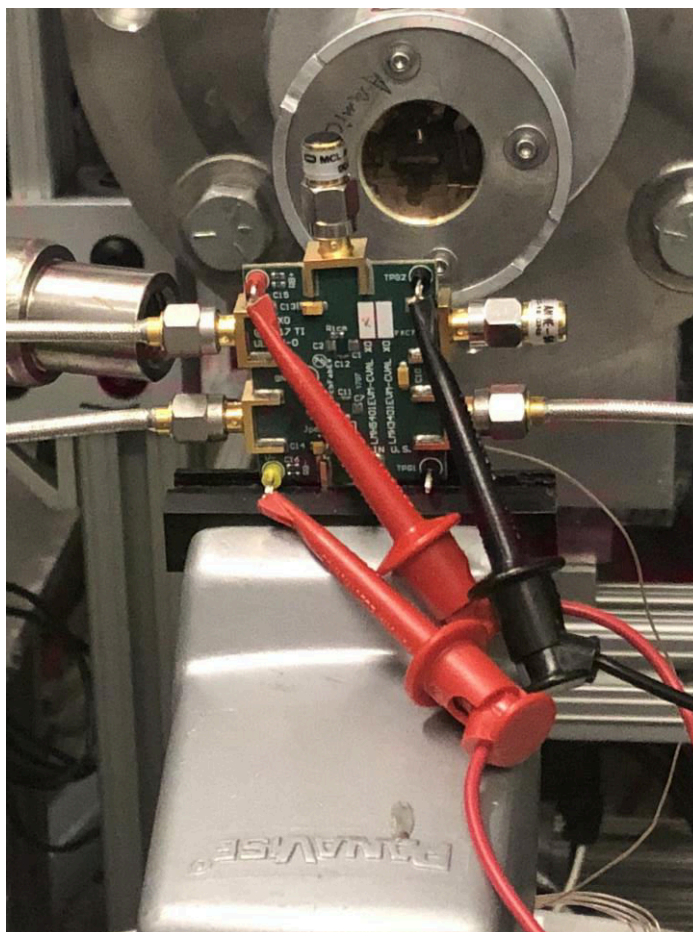
Figure 4-1. TRF0206-SP Evaluation Board Mounted in Front of the Heavy-Ion Beam Exit Port
