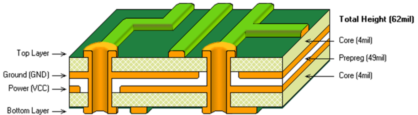
Figure 8. Board Stackup
