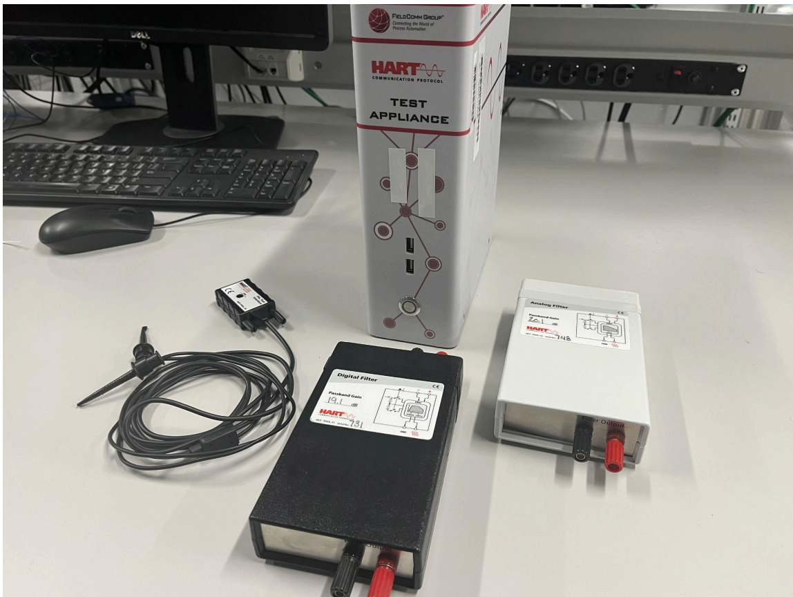
Figure 3-1. HART Test System Shown With an HCF_TOOL-31, HCF_TOOL-32, and an FSK Physical Test Interface
