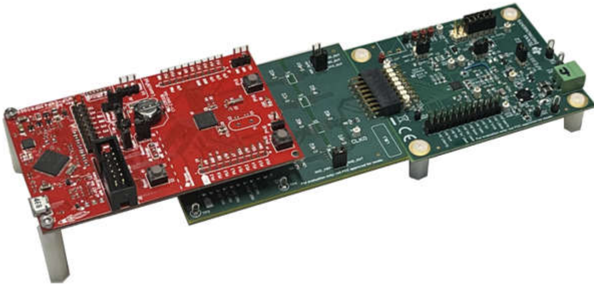
Figure 4-4. AFE882H1 Front-End Board With Digital Back-end Board and MSP430FR5969 Launchpad as a HART Transmitter
