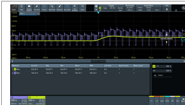
Figure 3-47. 2KV Surge at 230Vac input
