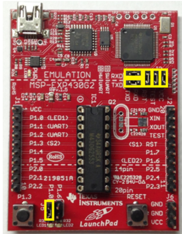
Figure 3. Proper Jumper Configuration on the LaunchPad
