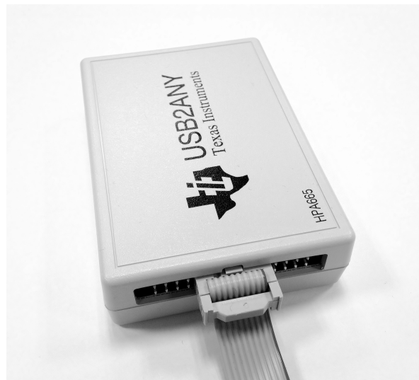
Figure 8. Ribbon Cable Connected to the Ten Middle Pins of the USB2ANY Interface Adapter
