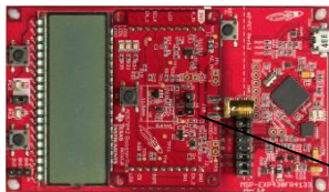
MSP430 LaunchPad & ADS7042 BoosterPack
