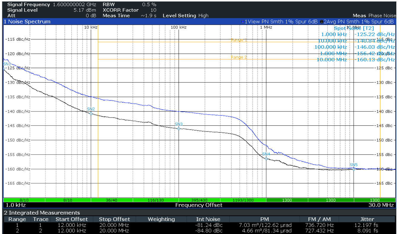
Figure 4-3. Divide-by-2 Mode Signal Analyzer Plot
