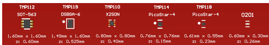
Figure 3. Device Size Comparison: Chip-Scale Devices (Topside View)
