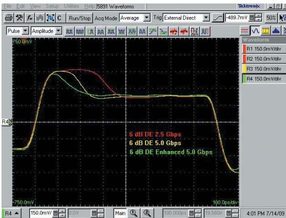
Figure 4. De-Emphasis Waveforms for 2.5G and 5.0G Operation
