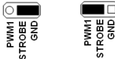
Figure 3. STROBE Jumper Settings
