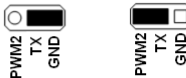
Figure 5. TX Jumper Settings
