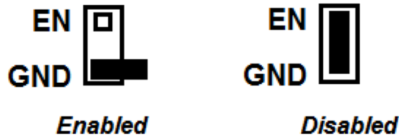
Figure 2. Enable Jumper Setting
