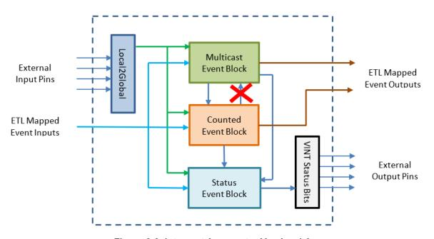
Figure 2-3. Interrupt Aggregator Version 1.0
