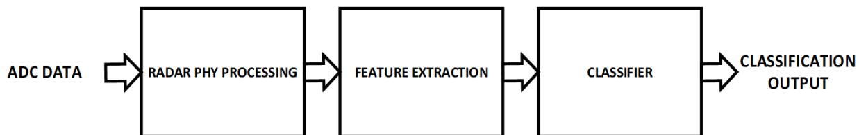
Figure 2-1. A Representative Radar Based Classification Chain
