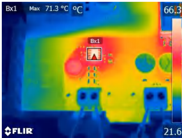
Figure 2-3. Buck: 24-V Input
