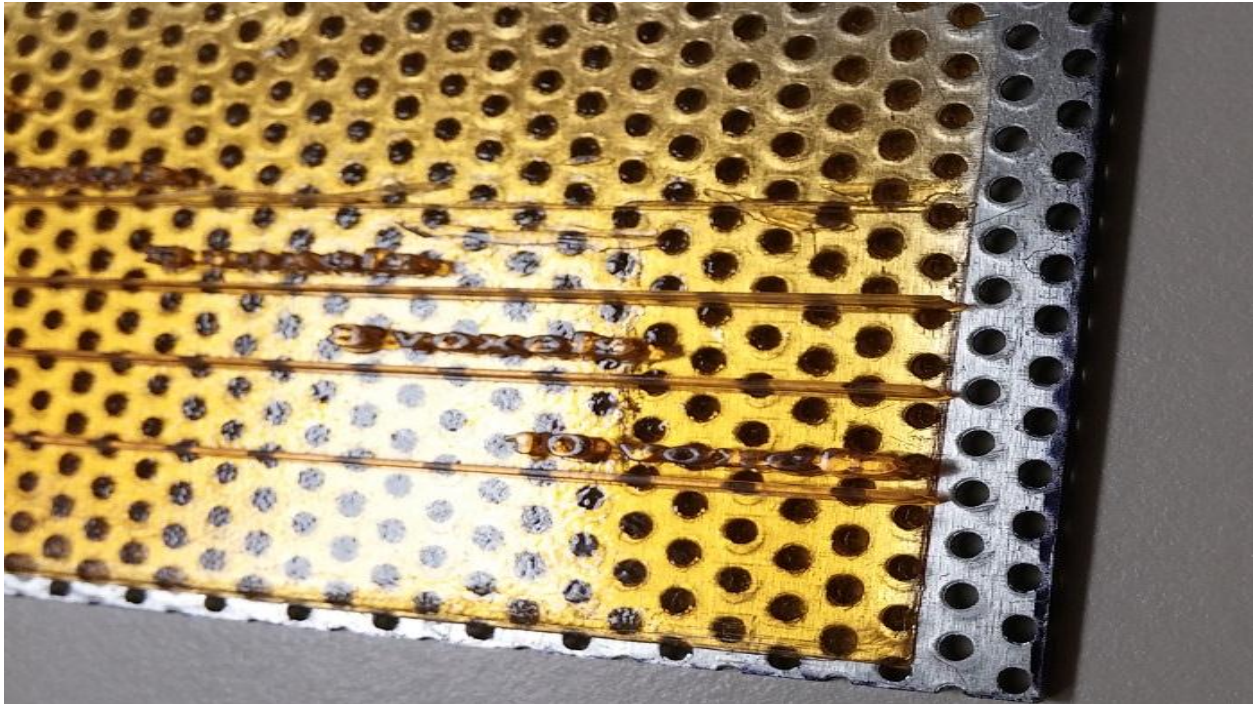
Figure 2. Determining minimum printable line width
