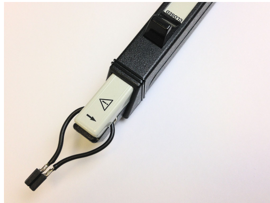
Figure 21. Combination of Current Probe With Self-Made Adapter for Primary Side Current Measurement
