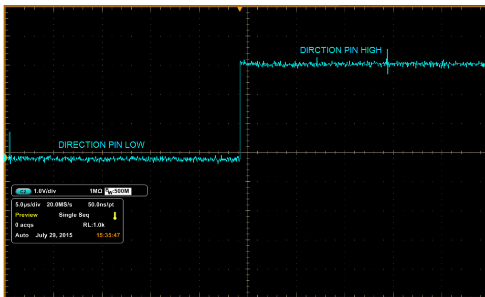
Figure 26. Phase State Change of MSP430G2553
