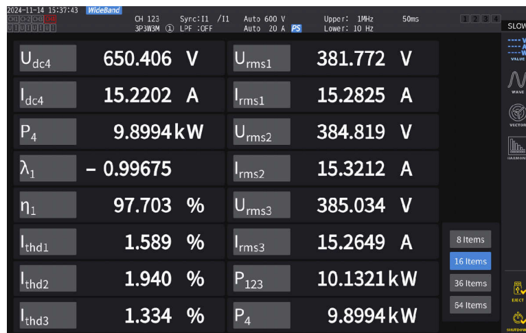
Figure 3-43. Power Analyzer Result Under 10kW Grid Power
