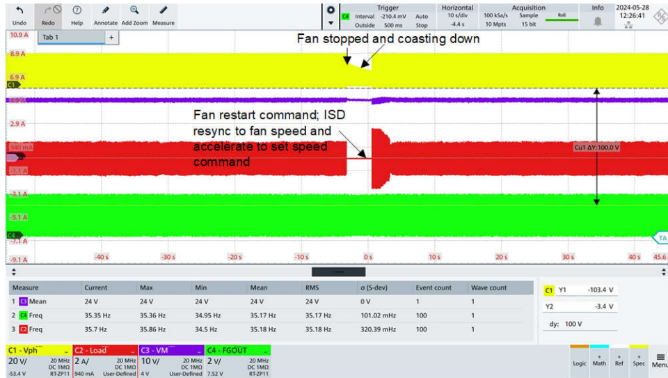
Figure 4-6. Forward Windmilling (High-Speed ISD Forward Resync)
