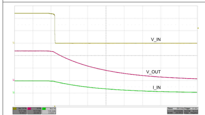
10-9. Power Fail With 24-Ω Load—Supports 1-A Load for 10-ms Power Fail
