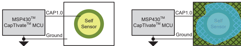
Figure 6. Self Capacitance Sensor With Hatched Filling Connected to Ground
