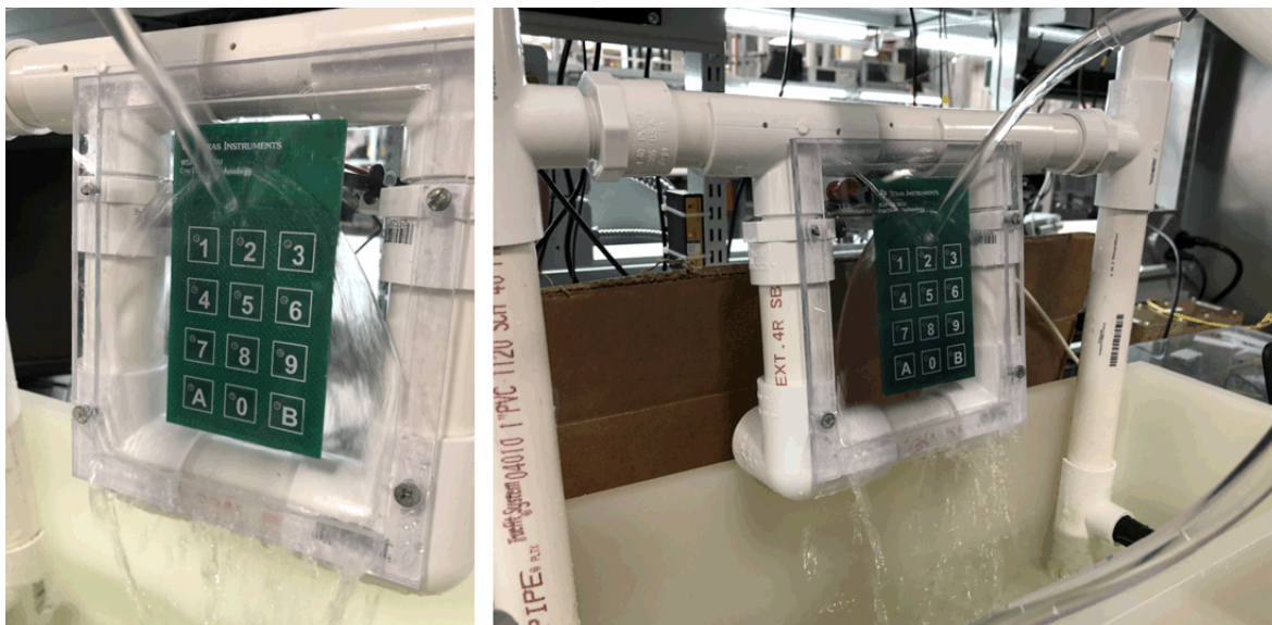
Figure 17. Continuous Water Flow Test Setup
