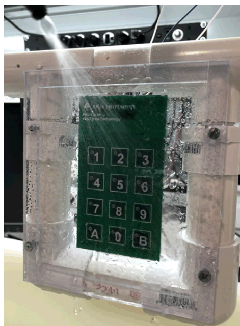
図 20. Continuous Water Spray Test Setup
