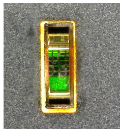
Figure 8-6. Image of FPCB With OPT4001-Q1 Mounted, Receiving Light Through the Cutout With a Rectangular Shape
