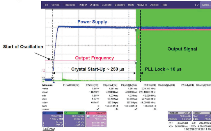
Figure 9-4. Crystal Oscillator Start-Up vs PLL Lock Time
