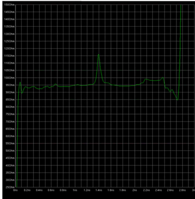
Figure 3-1. TDR Plot Example With Impedance Mismatch
