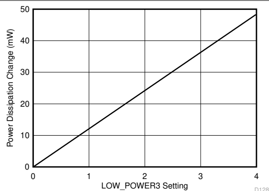
Figure 8-11. Power Dissipation Change vs LOW_POWER3 register setting
