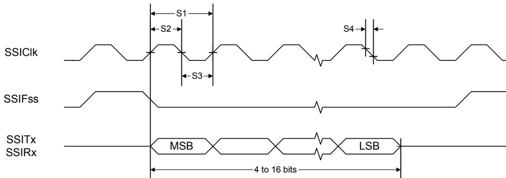
Figure 21-12. SSI Timing for MICROWIRE Frame Format (FRF=10), Single Transfer
