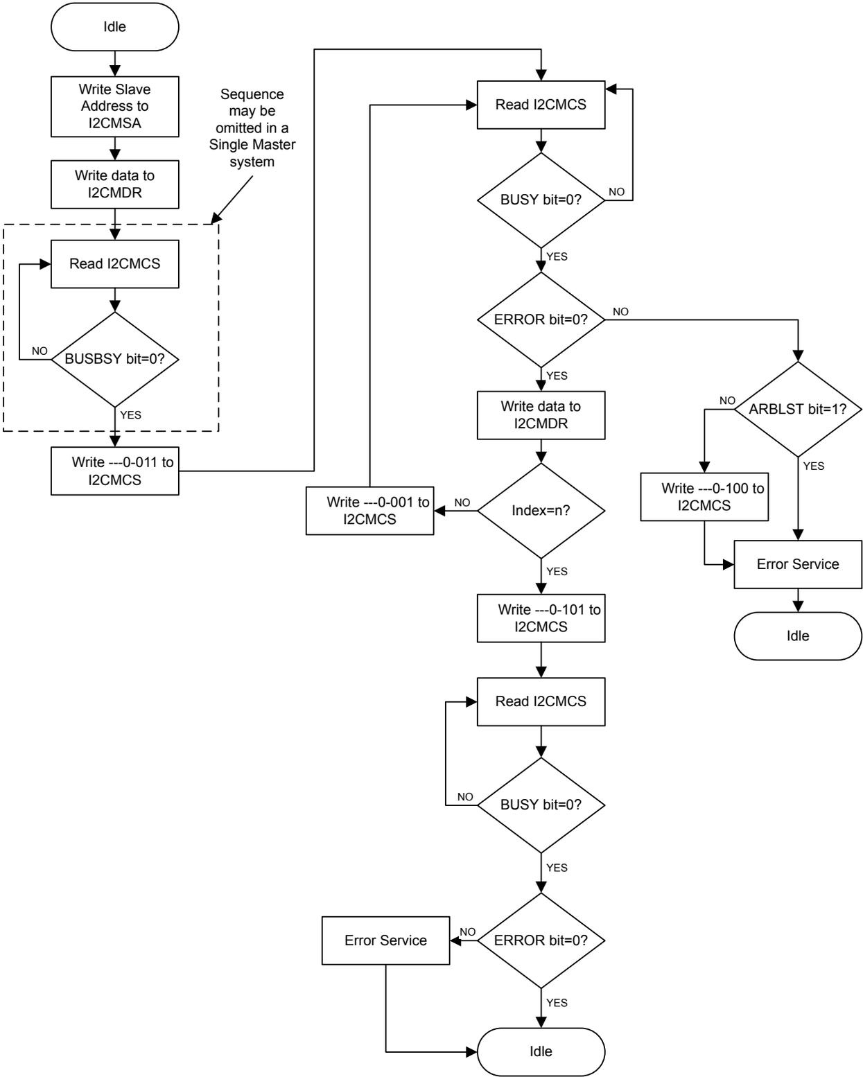
Figure 13-10. Master Burst RECEIVE
