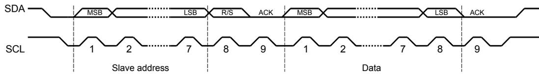
The first seven bits of the first byte make up the slave address (see Figure 13-5 on page 476). The eighth bit determines the direction of the message. A zero in the R/S position of the first byte means that the master will write (send) data to the selected slave, and a one in this position means that the master will receive data from the slave.
