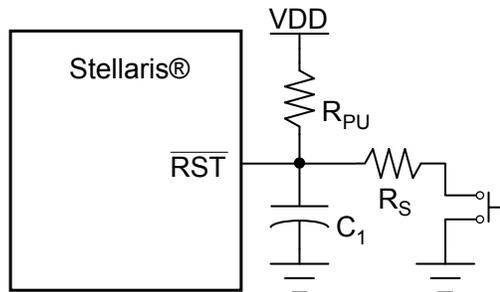
Typical  $R_{PU} = 10 \text{ k}\Omega$
