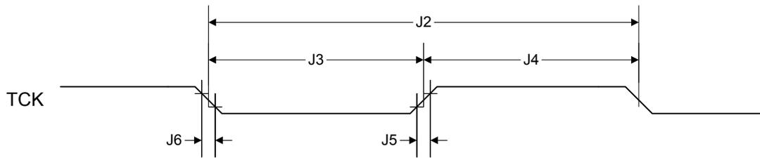
Figure 21-3. JTAG Test Access Port (TAP) Timing
