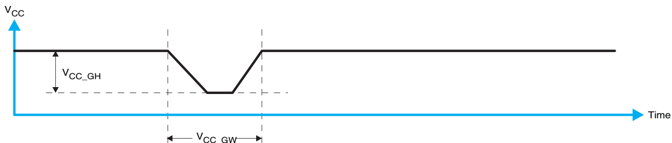
Figure 22. Glitch Width and Glitch Height
