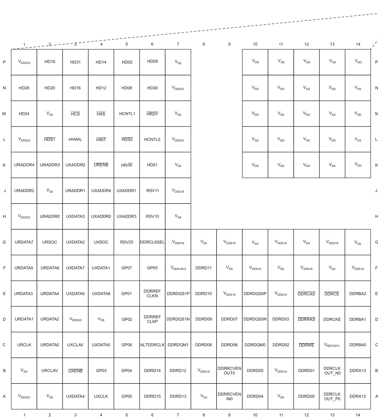
Figure 3-5. TCI648F Pin Map (Bottom View) [Quadrant D]
