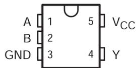
Figure 4-1. DBV or DCK Package (Top View)
