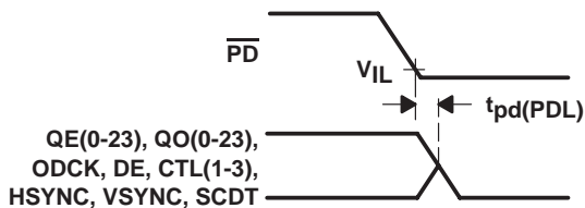
Figure 7. Delay From \overline{PD} Low to Hi-Z Outputs
