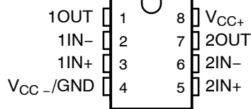
TLE2021 D, DB, JG, P, OR PW PACKAGE (TOP VIEW)
