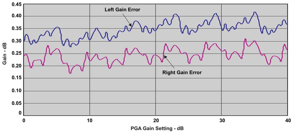
Figure 8. Single-Ended Gain Error
