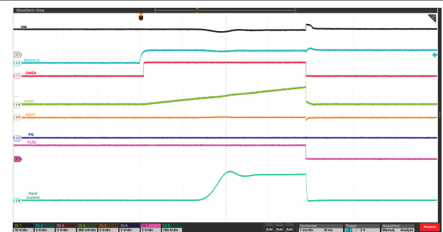
Figure 9-7. Power Up into Short: V_{IN} = 12 V, EN/UVLO Stepped Up From 0 V to 3 V, R_{IREF} = 40.2 k \Omega , R_{ILIM} on Each Device = 300 \Omega , and OUT Shorted to GND
