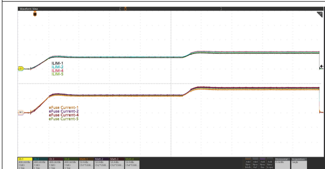
Figure 9-12. Circuit-Breaker Response (Current distribution among five devices in parallel): V_{IN} = 12\text{ V} , C_{ITIMER} = 22\text{ nF} , C_{LOAD} = 55\text{ mF} , R_{IMON} = 167\ \Omega , R_{IREF} = 40.2\text{ k}\Omega , and Load Current Stepped up From 300 A to 475 A for > 20 ms
