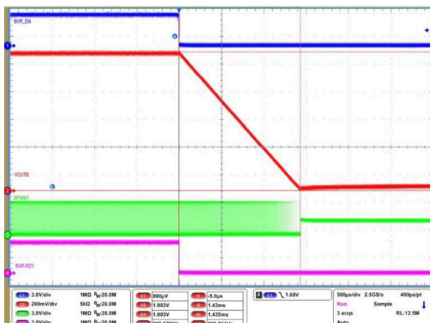
Figure 8-15. Soft-stop channel B (0 ms TOFF_DELAY)
