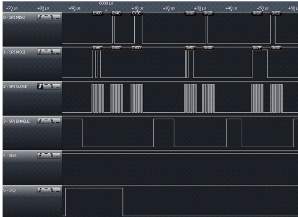
Figure 6-24. IRQ With One Byte in FIFO
