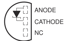
1.2 V ... LP (TO-92/TO-226) PACKAGE (TOP VIEW)
